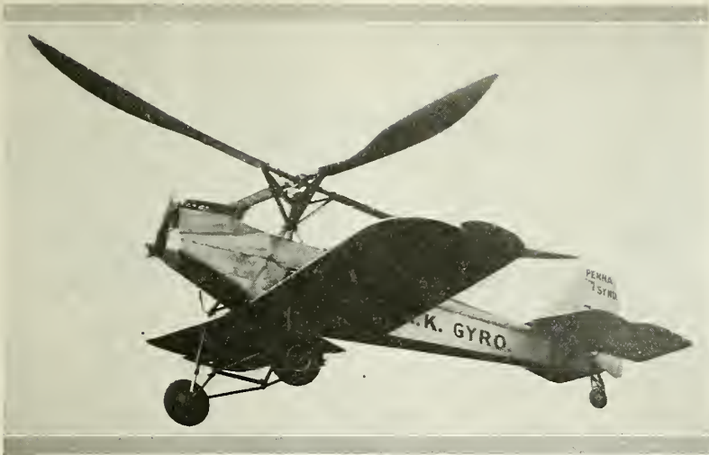
Flight test of the Wilford gyroplane with an 85 horsepower Cirrus engine
